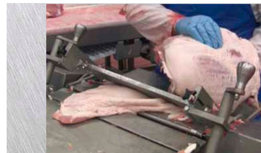
ESM 5550/1: Hand lever at the right and left side for rind thickness adjustment
