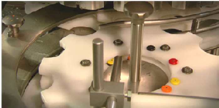
▲ Machine display. 10 pre-set product-format combinations. Also change part colour codes are shown.
